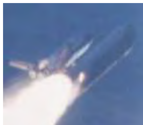
Challenger: escape de gas
